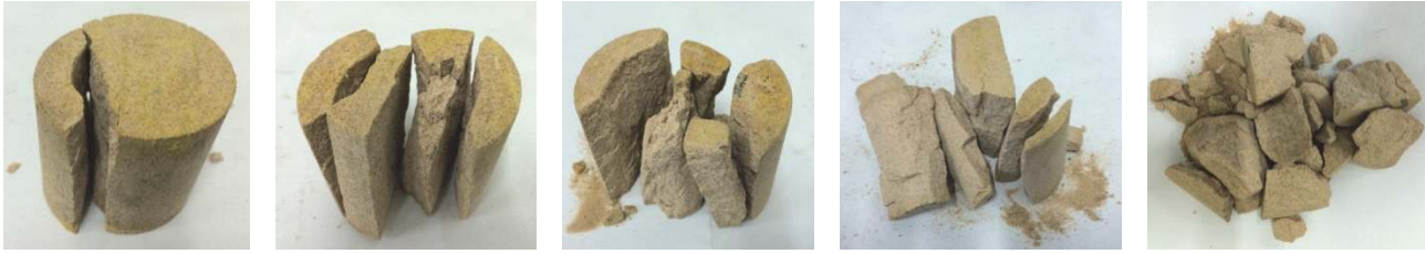
FIGURE 10: Failure forms under different freeze-thaw cycles.
