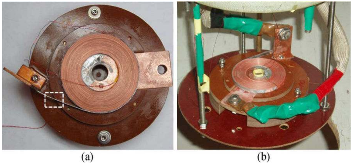
Fig. 1. (a) NI HTS single pancake test coil; (b) Test coil mounted in the LHe experimental setup.
