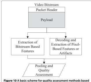
Figure 10 A basic scheme for quality assessment methods based on hybrid of NR-P- and NR-B-based approaches.
