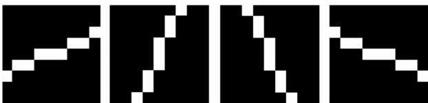
Fig. 1. Different configuration of pixels to define directional windows D_\theta , with N = 9 pixels and four equally spaced orientations \pi/8, 3\pi/8, 5\pi/8, 7\pi/8 . Note that periodicity is \pi , provided that \theta + \pi originates pixel arrays with the same PWD.
