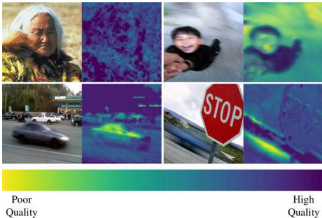
Figure 5. Spatial quality maps generated using the our proposed model. Left: Original Images. Right: Quality maps blended with the originals using viridis color.
