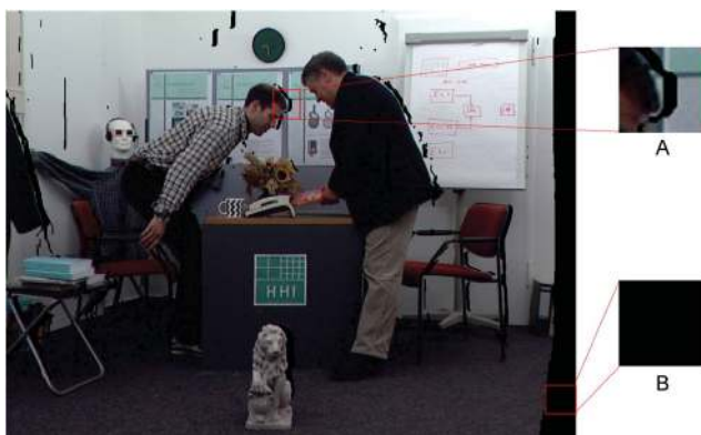
Fig. 3 Visual appearance of image patches containing geometric distortions. Patch A has partial holes, while patch B is dominated by holes. Compared to patch A, patch B is generally perceived as a higher quality image patch, if knowledge of geometric distortions in the whole image is not known.
