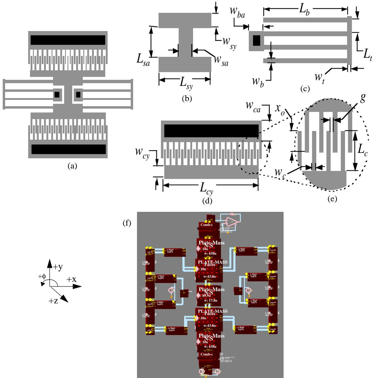
**Figure 23. Folded-Flexure resonators, (a) Layout view, parameterized microresonator elements (b) shuttle mass, (c) folded flexure, (d) comb-drive with N movable rotor fingers, (e) close-up view of comb-fingers (f) schematic view.**
