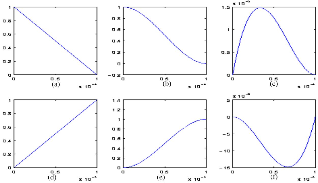
**Figure 9. Shape functions for unit displacements in the x, y, and  $\phi$  axes vs. position along the length of the beam, (a)  $x_a$  displaced, (b)  $y_a$  displaced, (c)  $\phi_a$  displaced, (d)  $x_b$  displaced, (e)  $y_b$  displaced, (f)  $\phi_b$  displaced.**
