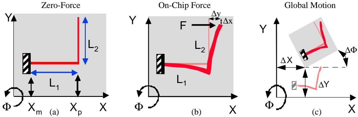
**Figure 2. Physical systems of a crab-leg structure. (a) Zero-Force system determining initial positions, (b) On-Chip forces causing on-chip displacements, (c) Global motion of chip causing changes in position.**
