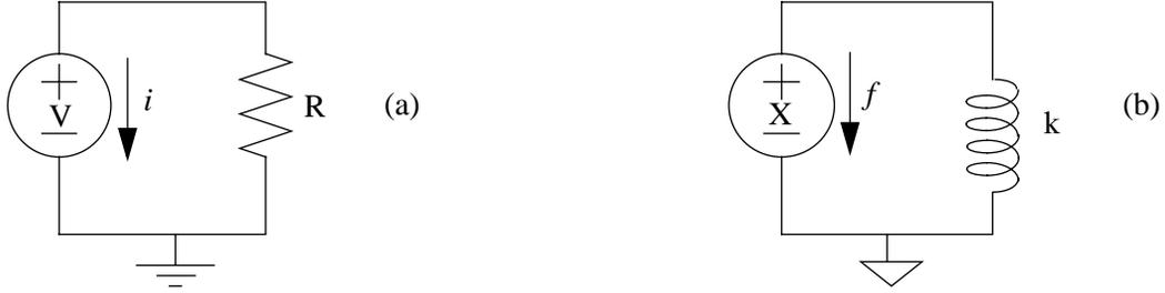
**Figure 4. (a) Voltage source connected to a resistor,  $R$ .  $V$  defines the voltage across the source, while the extra through variable,  $i$ , defines the current through the source such that the voltage is maintained. (b) Position source connected to a spring,  $k$ .  $X$  defines the position across the source, while the extra through variable,  $f$ , defines the force through the source such that the position is maintained.**
