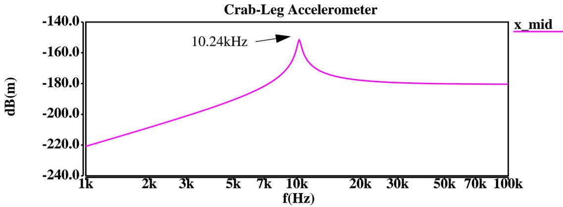
Figure 27. AC Analysis of the crab-leg accelerometer.
