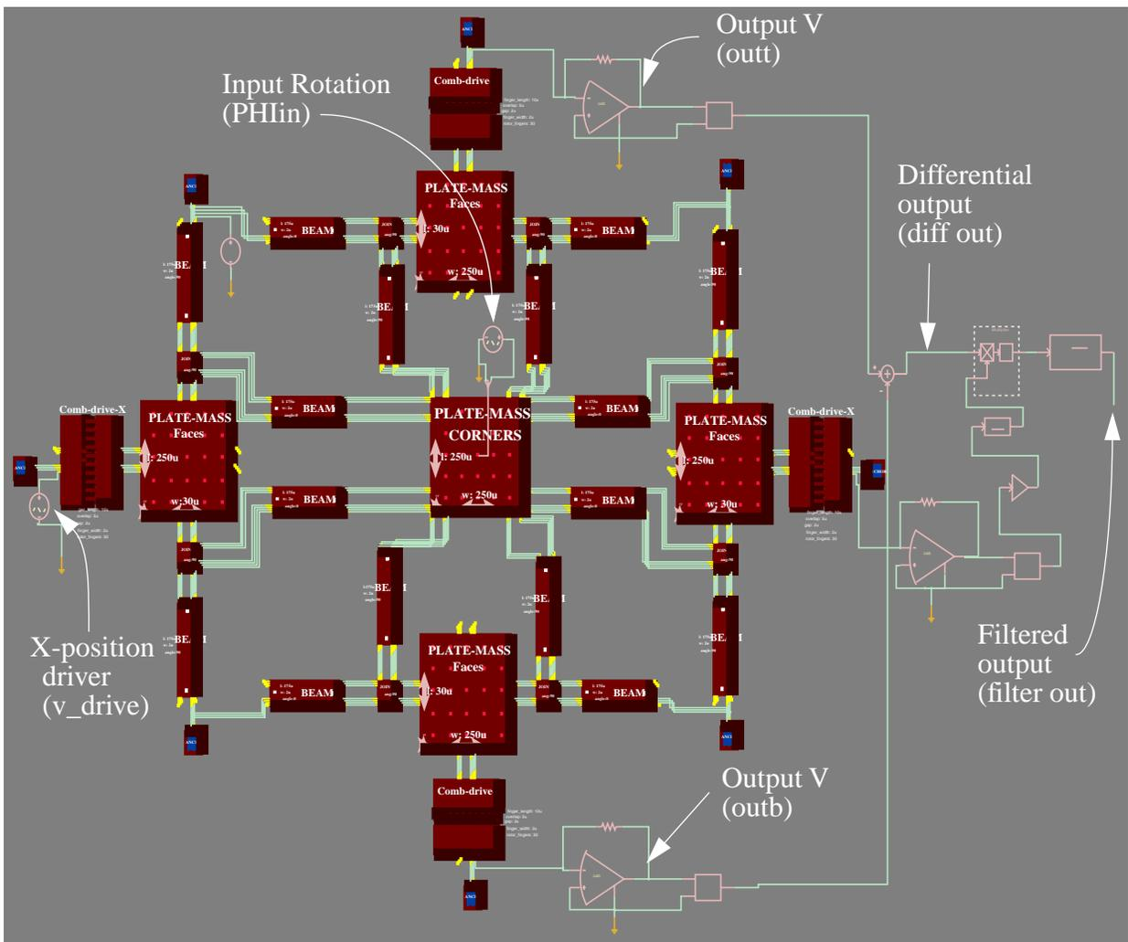
Figure 29. Equivalent schematic view of vibratory rate gyroscope.
