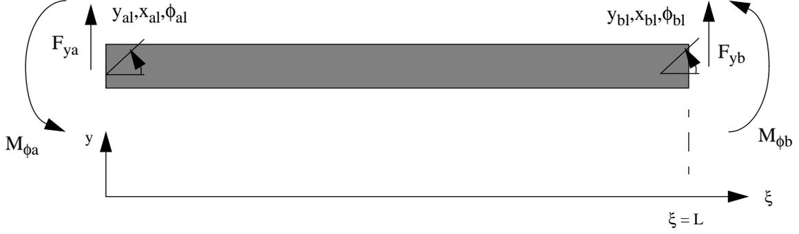
**Figure 8. General beam in local frame with shearing forces and bending moments.**
