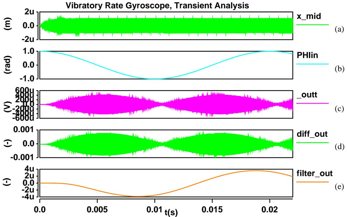
**Figure 30. Transient analysis of vibratory rate gyroscope, (a) X axis motion due to input driving voltage ( $v\_drive$ ), (b) external rotation ( $PHlin$ ), (c) top combdrive's electrical output ( $outt$ ), (d) differential output signal ( $diff\_out$ ), (e) demodulated, and filtered output ( $filter\_out$ ).**
