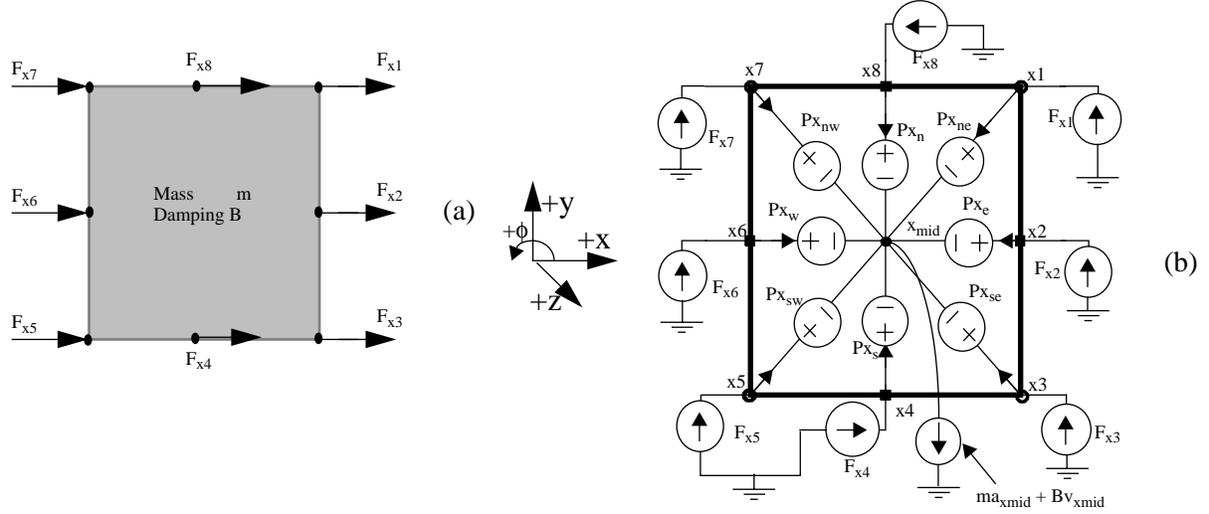
**Figure 12.(a) Mechanical element with applied forces,  $F_{x_i}$ ,  $i = 1$  to  $8$ ,
