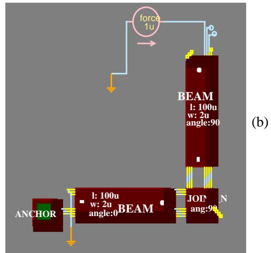
Figure 19. Crab-Leg Flexure, with force in the positive x direction, (a) Layout View, (b) SABER schematic view.
