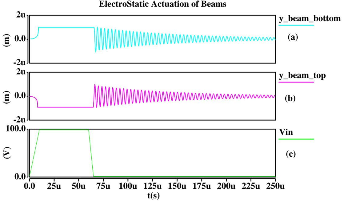
**Figure 25.** Transient analysis of comb finger snapping and release due to electrostatic actuation, (a) y-displacement at the left corner of the bottom beam, (b) y-displacement at the right corner of the top beam, (c) input voltage.
