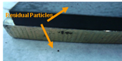
Fig. 15. Residual particles and films.
