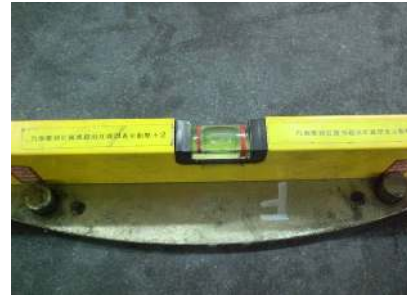
Fig. 13. Warping/deformation check for rubbing plates.
