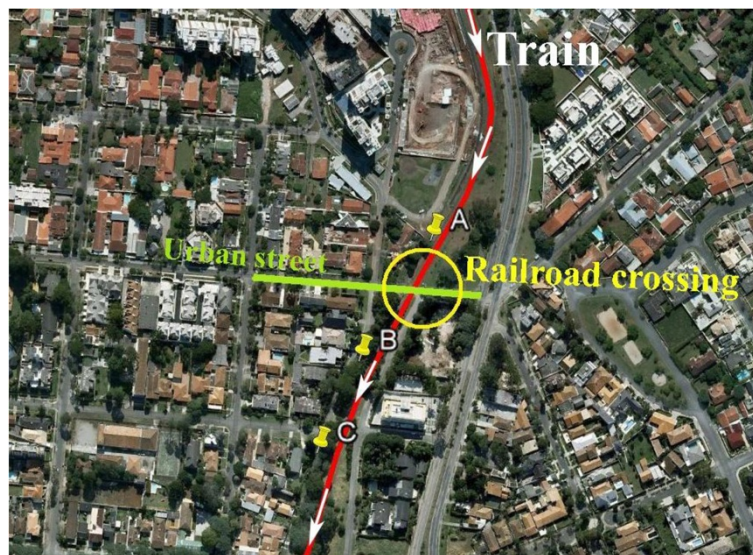
Figure 7 Measurement points along the railway line: A – Train passing with horn blowing, B – Train passing without horn blowing, C – Ambient noise without train passing.
