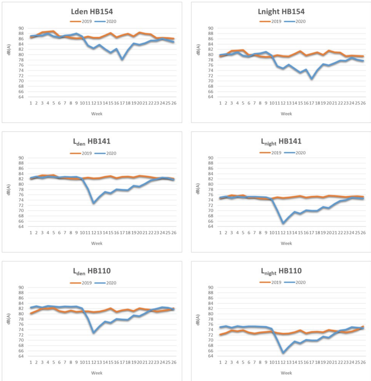
Figure 15: Noise trend retrieved from the three monitoring devices installed along the road stretch in the pilot area of Rome
