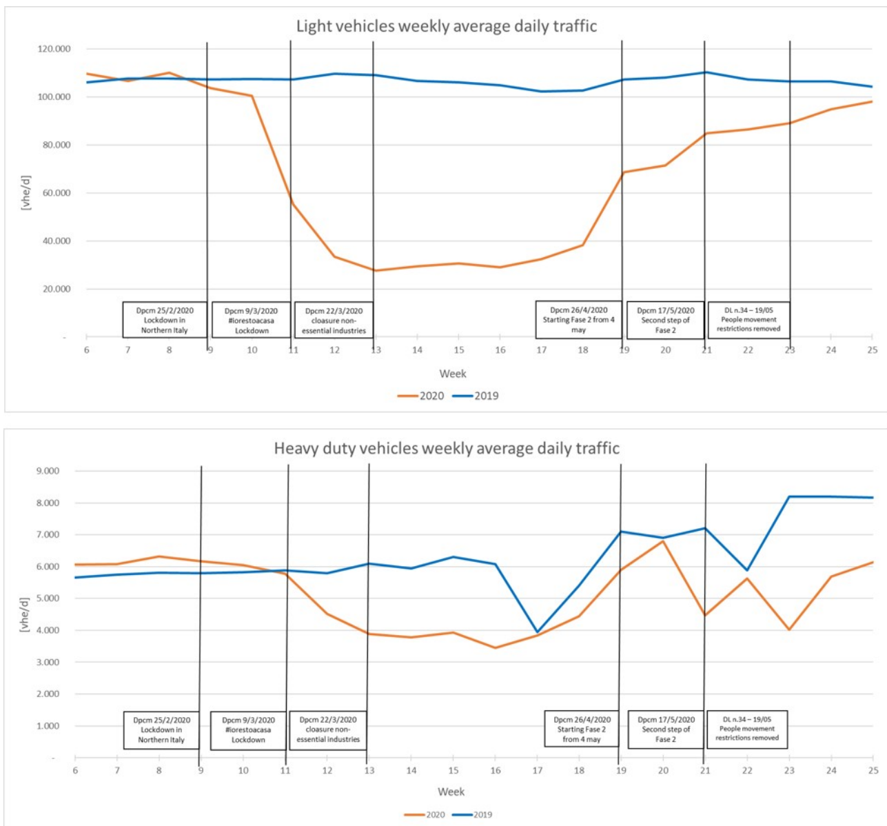
Figure 11: Weekly average daily traffic on the road stretch of the A90 under investigation related to light and heavy duty vehicles
