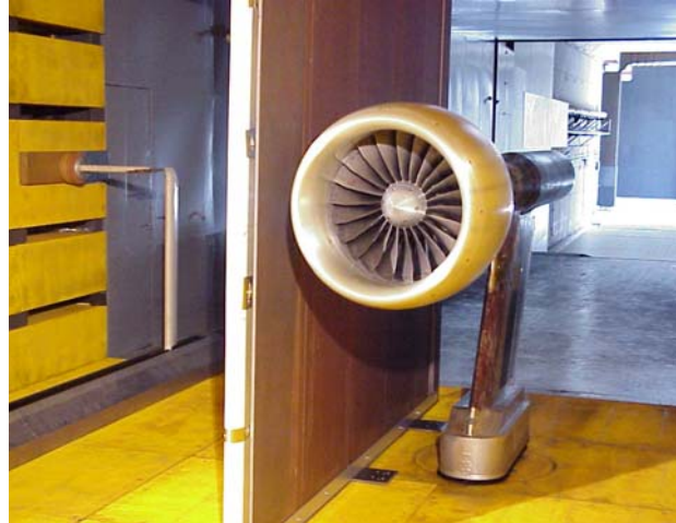
Figure 8.—Photograph of the research fan stage with the acoustic barrier wall in place.
