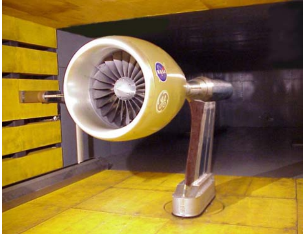
Figure 7.—Photograph of the research fan stage installed in the 9- by 15-Foot LSWT.
