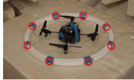
Fig. 5: Sensing unit consisting of an AR.Drone, a RASP-24 signal processing unit and a microphone array, which had eight microphones at the locations marked by red circles.
