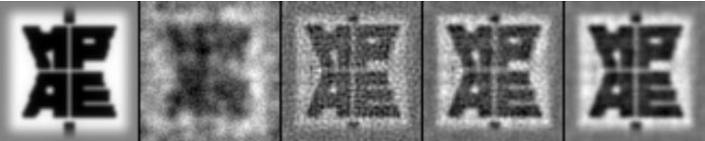
Fig. 3. Test reconstructions of an artificial intensity distribution, from the left to the right this figure represents the original intensity distribution, a typical speckle interferogram affected by seeing and noise, and the reconstructions with the optimum filter NF_2 , the phase number filter NF_3 , and the combined filter NF_2 \cdot NF_3 ; again, each picture is scaled individually
