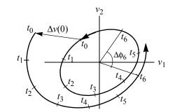
Consider plotting two state variables for an oscillator against each other, as shown in Figure 7. In steady state, the trajectory is a stable limit cycle, *v*. Now consider perturbing the oscillator with an impulse and assume that the response to the perturbation is  $\Delta v$ . Separate  $\Delta v$  into amplitude and phase variations,
