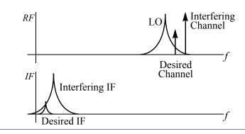
Similarly, phase noise in the signal produced by a nearby transmitter can interfere with the reception of a desired signal at a different frequency produced by a distant transmitter.
