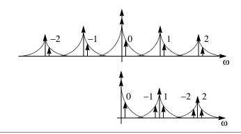
Because of the translation of replicated copies of the same noise source, noise separated by  $kf_0$  is generally correlated. Remember that noise folds across DC, so noise in upper and lower sidebands will be correlated. Consider the top of Figure 3 where noise is
