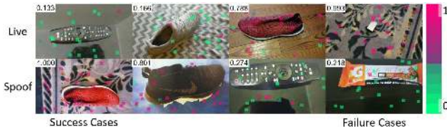
Figure 6. Illustration of GOLab-based anti-spoofing, with 2 success (left) and 2 failure (right) cases for live (top row) and real spoof (bottom row) using 20 patches per image. The color bar shows the output range of the network: 1 is spoof and 0 is live. The score at the top left corner is the average of all patches.
