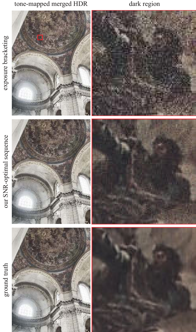
Figure 5. HDR merging results for the Nancy church scene, using capture sequences described in Fig. 4(top). We used a high-quality HDR image as ground truth, and synthetically generated the required input images by applying our image formation model (Sec. 2) with the noise parameters of the Canon 1D Mark III. Top: Reference 3-shot exposure bracketing sequence, with images 2 stops apart. Middle: Our optimal 3-shot capture sequence, maximizing worst-case SNR in the same time budget. Bottom: Ground truth. Please see electronic copy for better tone reproduction.
