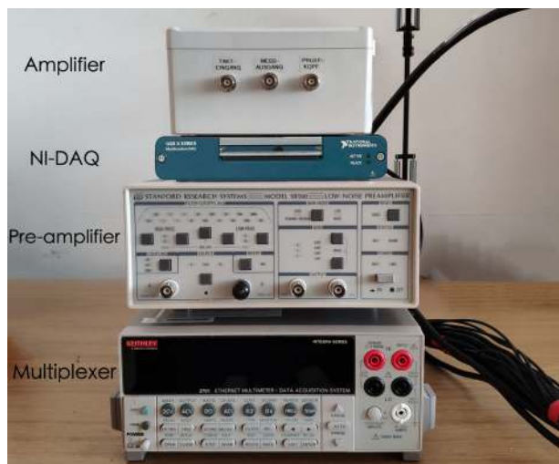
Fig. 7 Setup of data acquisition devices
