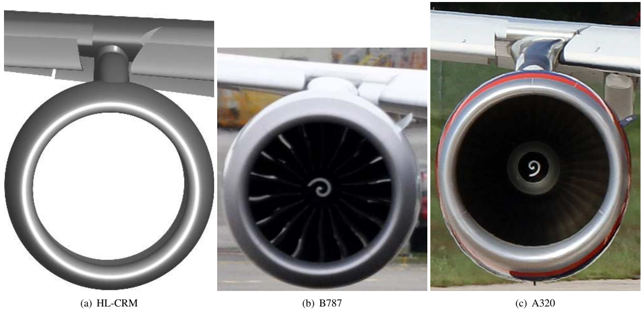
Figure 11. Comparison of the pylon / wing junction region between the HL-CRM, B787, 57 and A320. 58 Photos obtained from Wikimedia Commons and reproduced under the Creative Commons Attribution-Share Alike 2.0 Generic license.
