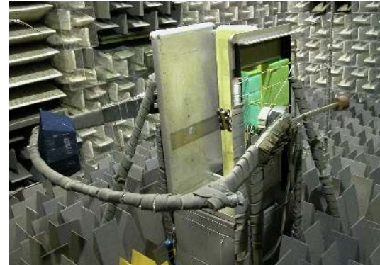
Figure 3. Model mounted in QFF for flyover viewing.
