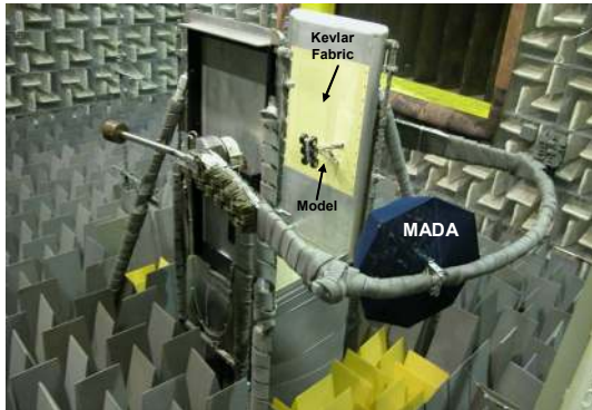
Figure 2. Model mounted in QFF for sideline viewing.
