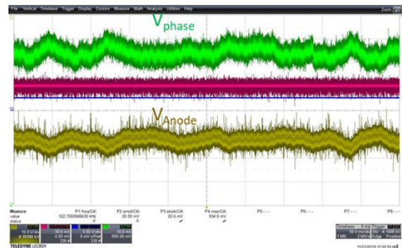
FIGURE 15. Long-term drift of the phase (green) and the anode voltage (yellow), which is exact replication of the anode-voltage variation to maintain the anode-current at a constant value.
