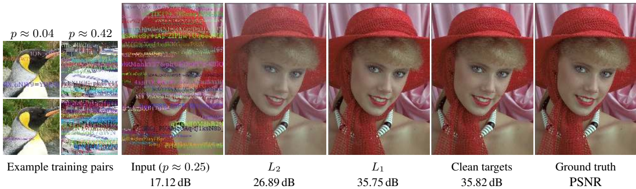
Figure 3. Removing random text overlays corresponds to seeking the median pixel color, accomplished using the L_1 loss. The mean ( L_2 loss) is not the correct answer: note shift towards mean text color. Only corrupted images shown during training.
