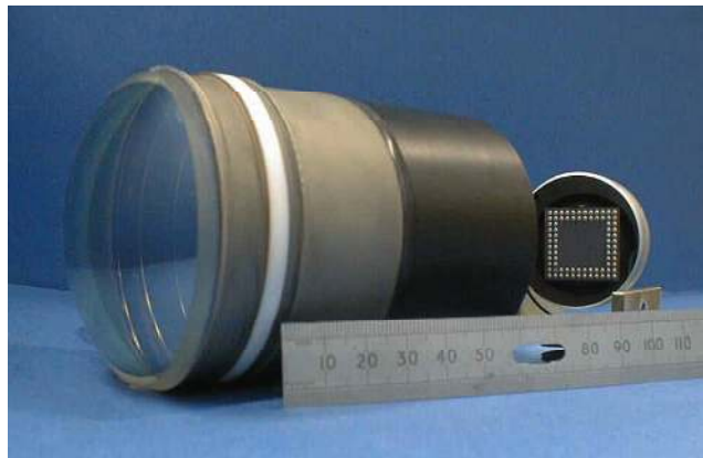
Fig. 13. Photograph of the 72:18 mm HPD prototype tube manufactured by DEP for the LHCb-Ring Imaging Cherenkov (RICH) Detector project equipped with a 61-pixel anode and read out externally with the IDE VA2 analysis chip. ( http://www.cern.ch/~gys/LHCb/PixelHPDs.htm )
