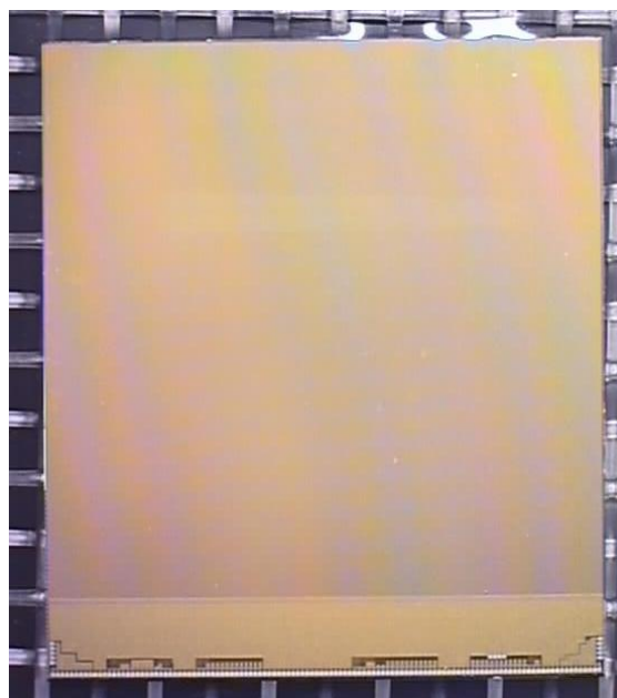
Fig. 6. Image of input face of Medipix2 chip. The dimensions are 1.6 cm high and 1.4 cm wide. The active area has 256x256 pixels and is abutable on 3 sides.
