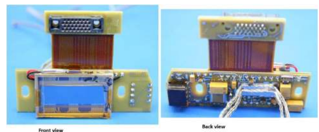
Fig. 13. Flight spare detector board.
