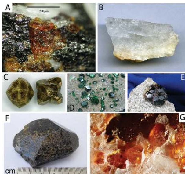
FIGURE 1. Photographs of representative garnet supergroup minerals illustrating the diversity in appearance exhibited by the supergroup. (a) Holtstamite, formula \{Ca_3\}[Al,Mn^{3+}](Si_2)(\square)O_8(OH)_4 , as a yellow brown crystal between grains of Mn- and Cu-rich vesuvianite (purplish black) and calcite (white) in the holotype specimen from Wessels Mine, South Africa. Swedish Museum of Natural History specimen no. 19960380. Photo by U. Hålenius. (b) Cryolithionite, end-member formula \{Na_3\}[Al_2](Li_3)F_{12} : a transparent, colorless single grain in yellowish-white fine-grained cryolite. Specimen size is 4.5 \times 2 \times 1.7 cm. From the type locality, Ivigtut Cryolite deposit, Ivittuut (Ivigtut), Kitaa, Greenland. Pavel M. Kartashov collection and photograph. (c) Grossular, end-member formula \{Ca_3\}[Al_2](Si_3)O_{12} : a trapezohedron \{211\} , 3.5 cm across on the left and crystals in a cyclic intergrowth on the right, from the type locality, Wiluy River, Sakha-Yakutia Republic, Russia. The distinctive brown color is due a 30–50 \mu m zone of brown andradite a short distance under the crystal faces. Evgeny and Irina Galuskin collection and Evgeny Galuskin photograph. (d) Uvarovite, end-member formula \{Ca_3\}[Cr_3^{3+}](Si_3)O_{12} : green dodecahedral crystals on chromite, from the type locality, Saranovskii Mine, Permskaya Oblast, Middle Urals, Russia. Largest crystal is 4 mm across. Museum of the Faculty of Earth Sciences, University of Silesia, no. WNoZ/M/9/19. Evgeny Galuskin photograph. (e) Almandine, end-member formula \{Fe_3\}[Al_2](Si_3)O_{12} : a crystal group 2.5 cm across on granite, Mount Lady Franklin, Barnawartha, Victoria, Australia. Museum Victoria registration no. M34200. Frank Coffa photograph. (f) Schorlomite, end-member formula \{Ca_3\}[Ti_2](SiFe_3^{3+})O_{12} : an incomplete crystal from the type locality, Magnet Cove, Hot Spring County, Arkansas. E.S. Grew collection and photograph. (g) Manganberzeliite, end-member formula \{Ca_2Na\}[Mn_2^{2+}](As_3^+)O_{12} , from the type locality, Långban, Sweden. The largest crystals are 3 mm across. Swedish Museum of Natural History specimen no. 19170722. M. Cooper photograph.
