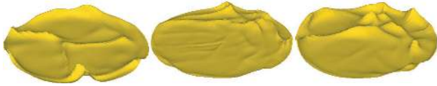
Figure 10. Temperature isosurfaces for T = 0.8 . The leftmost panel is for the non-Boussinesq case when all properties are allowed to depend on temperature; the middle panel corresponds to viscosity alone being a function of temperature; the right panel corresponds to the case for which the expansivity alone is a function of temperature.
