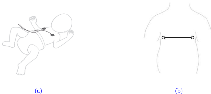
Figure 2.7 Neonatal impedance pneumography (IP). The IP electrodes are positioned bilaterally across the infant’s chest and below the insertion of the diaphragm [Di Fiore, 2004]. (2.7a) Whole body view. (2.7b) Front view.
