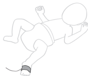
Figure 2.14 Neonatal pulse oximetry. In this scenario, the pulse oximetry is placed inside a pad conforming to the shape of the infant's foot.
