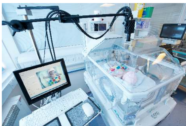
Figure 3.5 Data acquisition apparatus. Monitoring equipment imaging a mannequin inside the study incubator in the Oxford Neonatal Unit.
