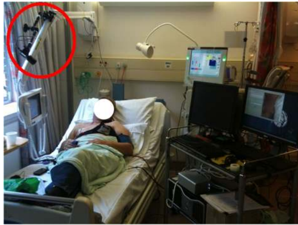
Figure 5. A typical dialysis data collection set-up. The red circle shows the location of the video camera. A pulse oximeter is attached to the patient's finger on the right hand. The Equivalital EQ-02 LifeMonitor is located on the patient's chest. Consent was obtained from the patient to use the image.
