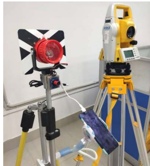
Figure 3. Simple hardware system for close - range photogrammetry
