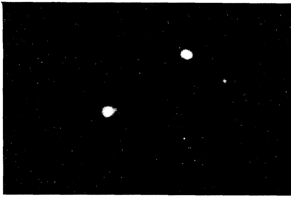
Fig. 5. Glare spots on the droplet midplane at an observation angle of \theta_0 = 90 \pm 1^\circ . The droplet diameter was 3.5 mm, and the exposure time was 120 s.
