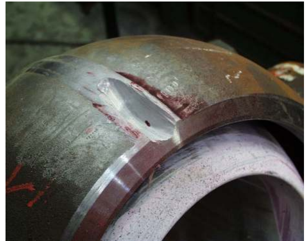
Figure 5 : the defect detected by TOFD is made evident by grinding and dye penetrant inspection
