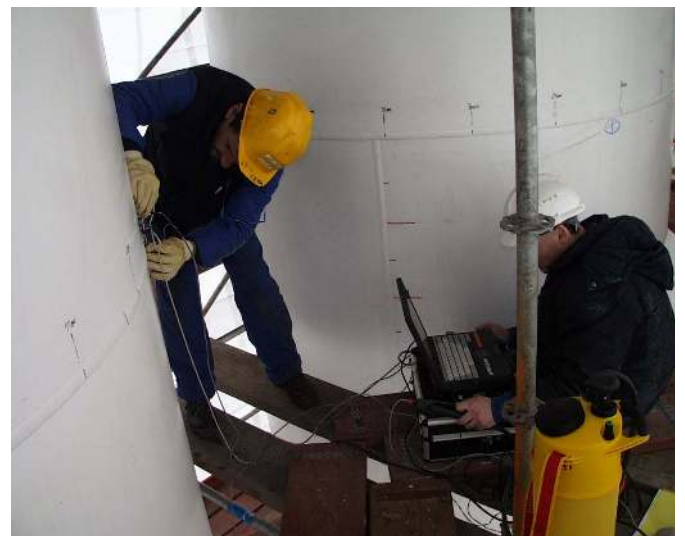
Figure 9 : Toftd control operated on site : producing an « ultrasonic film of the weld »
