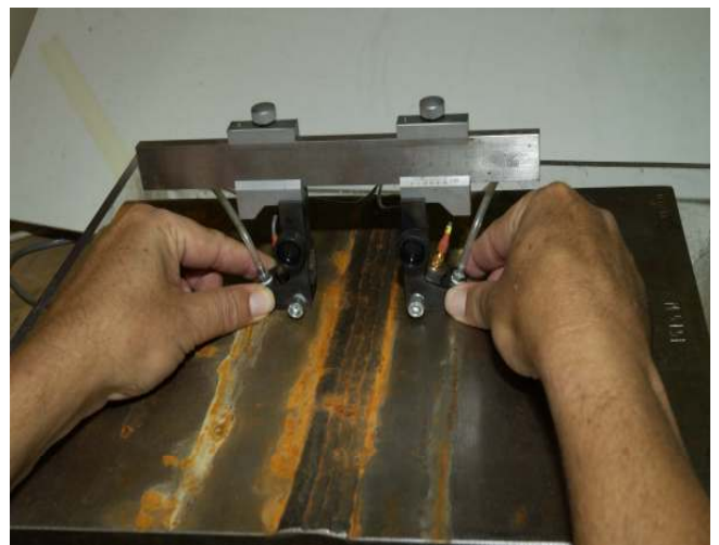
Figure 3: Tofd transducers for welding inspection
