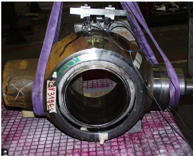
Figure 2: Tofd weld inspection on valve
