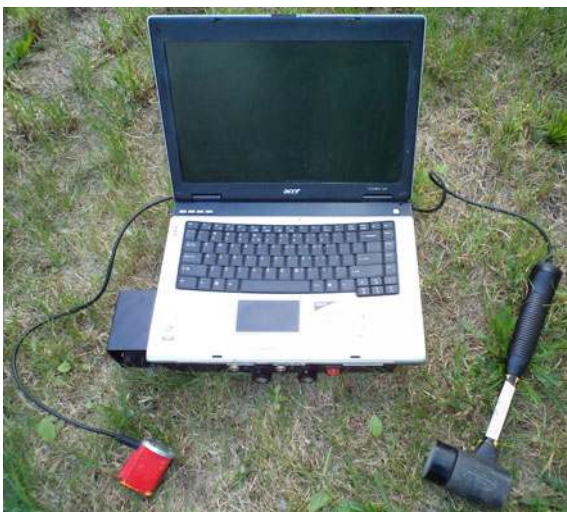
Fig. 3. Test equipment used in non-destructive acoustic impulse response technique
