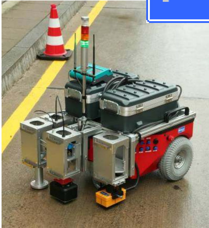
Self navigating Robot for horizontal surfaces (Park decks)
