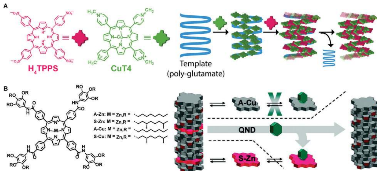
Fig. 11 Template assisted self-assembly. (A) A tetracationic porphyrin (CuT4) is assembled on a polyglutamate template, afterwards, a tetraanionic porphyrin (H 4 TPPS 4 ) is assembled in the pre-templated aggregates. Removing the template, the formed assemblies were retained. (B) Chiral porphyrin assemblies were formed via a “sergeant-and-soldier” strategy, removal of the sergeant Zn–porphyrin by axial ligation results in the kinetically trapped assemblies of Cu–porphyrin. Adapted from ref. 48 with permission from the American Chemical Society, copyright 2010.
