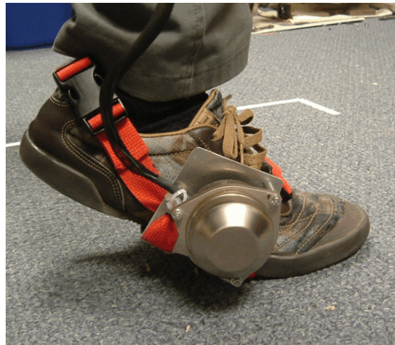
Figure 1: BAE SiIMU01 Inertial measurement unit (IMU) mounted to the foot of a walking subject. Of course, this IMU is too large for most practical uses. Our intention is to implement the PDR system with a much smaller IMU in the near future.
