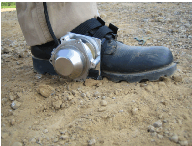
Figure 1: The University of Michigan’s two IMUs mounted to boots. (a) The SiIMU used in our earlier proof-of-concept prototype; (b) the small-sized nIMU, described in this paper.
