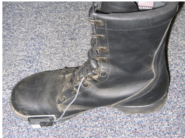
Figure 1: The University of Michigan’s two IMUs mounted to boots. (a) The SiIMU used in our earlier proof-of-concept prototype; (b) the small-sized nIMU, described in this paper.
