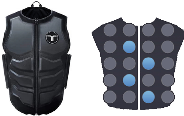
Fig. 2. Wearable haptic suit with a double matrix of vibrating motors for vibrotactile feedback.
