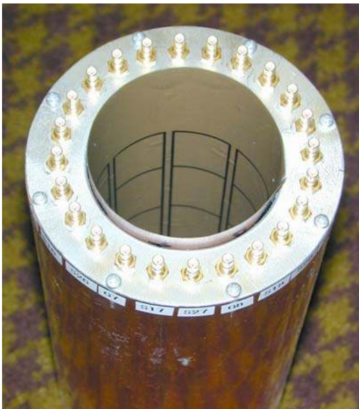
Figure 3. Photograph of sensor showing internal electrodes and connectors
