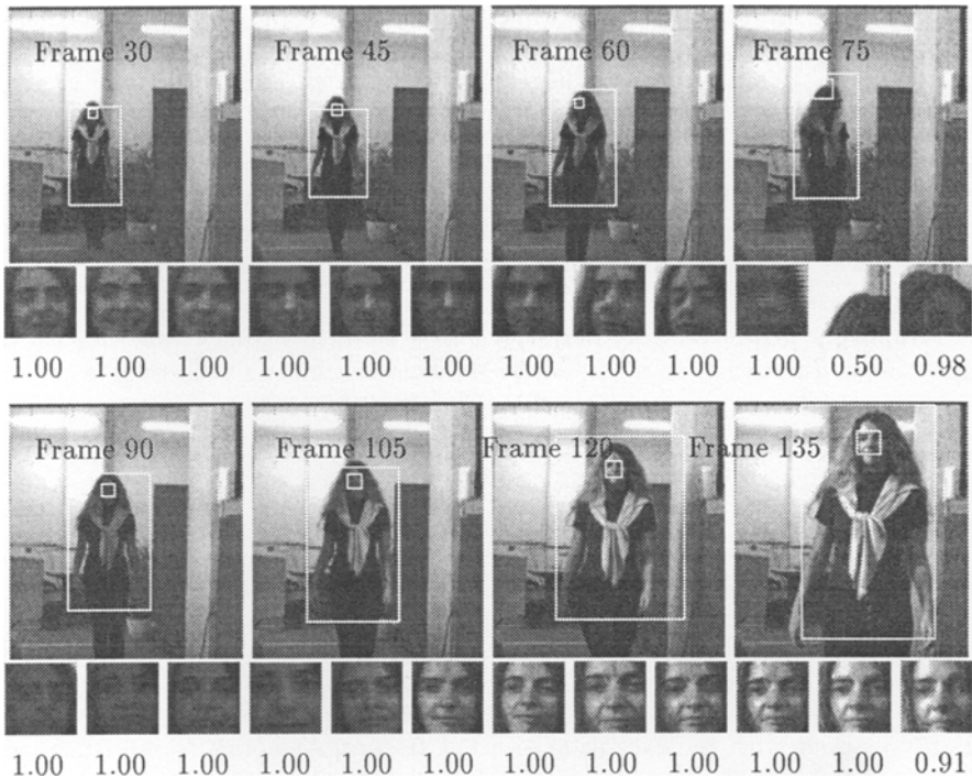
Fig. 2. A girl is tracked for recognition as she approaches the camera. Bounding boxes for the Kalman filtered motion cluster and the associated tracked face region are shown overlaid on every 15 th frame. The face is shown centred and normalised in scale every 5 th frame. The confidence values for each segmented face are also given.
