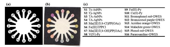
Fig. 1 The proposed paper based microfluidic sensor: a the design, b the image, and c the location of sensing elements
