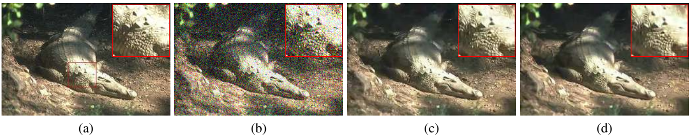
Figure 5. Color image denoising. (a) Original image, (b) Noisy image corrupted with Gaussian noise ( \sigma = 50 ); PSNR = 14.15 dB. (c) Denoised image using \text{CNLNet}_{5 \times 5}^3 ; PSNR = 26.06 dB. (d) Denoised image using CBM3D [7]; PSNR = 25.65 dB.
