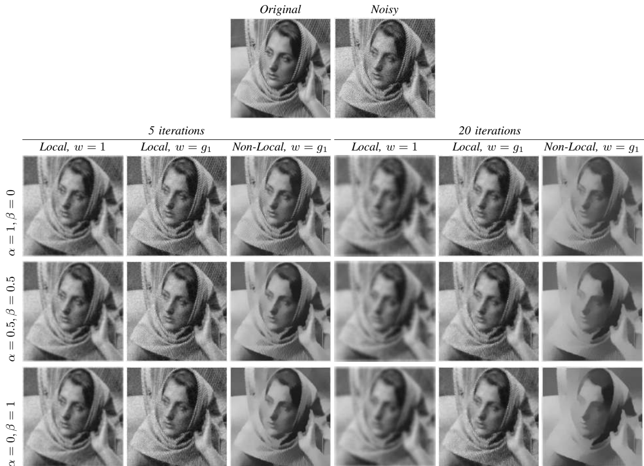
Fig. 1. Scalar image simplification on a gray level image with different parameters values of \alpha, \beta and different weight functions in local and non-local configurations, with 5 or 20 iterations. First row shows results for \alpha = 1, \beta = 0 ( \Delta_\infty ). Second row shows results for \alpha = 0.5, \beta = 0.5 . Finally, third row shows results for \alpha = 0, \beta = 1 ( \Delta_2 ). See text for more details.
