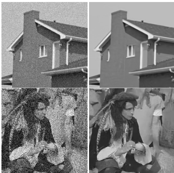
Figure 2. Qualitative evaluation of our denoising method with standard images. Left: noisy images. Right: restored images. Note that we reproduce the original brick texture in the house image ( \sigma = 15 ) and the hair texture for the man image ( \sigma = 50 ), both hardly visible in the noisy images. (The details are better seen by zooming on a computer screen.)
