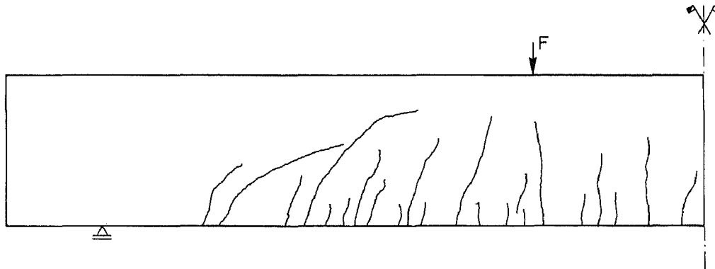
Figure 7 Experimentally observed crack pattern at impending failure
