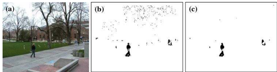
Fig. 5 Enforcing spatial consistency: a original frame b Detected foreground regions by applying thresholds directly on the estimated probability. c Detected foreground regions by applying threshold on median of probabilities in a neighborhood
