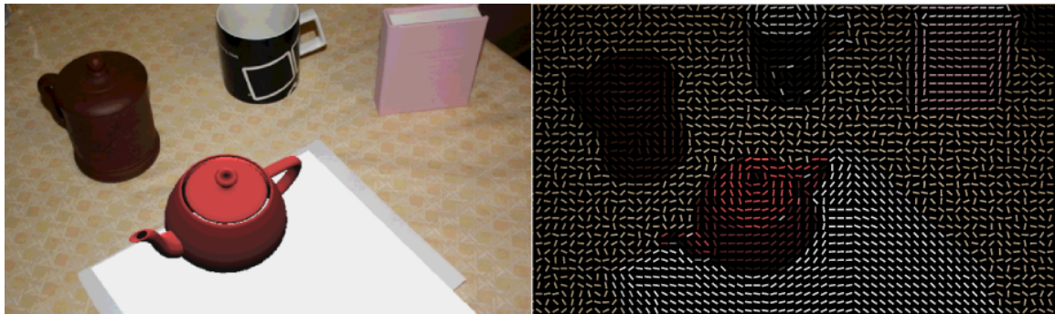
Figure 16: Tensor field visualization of an AR frame. There are a virtual teapot, two real cups and an album on the table.
