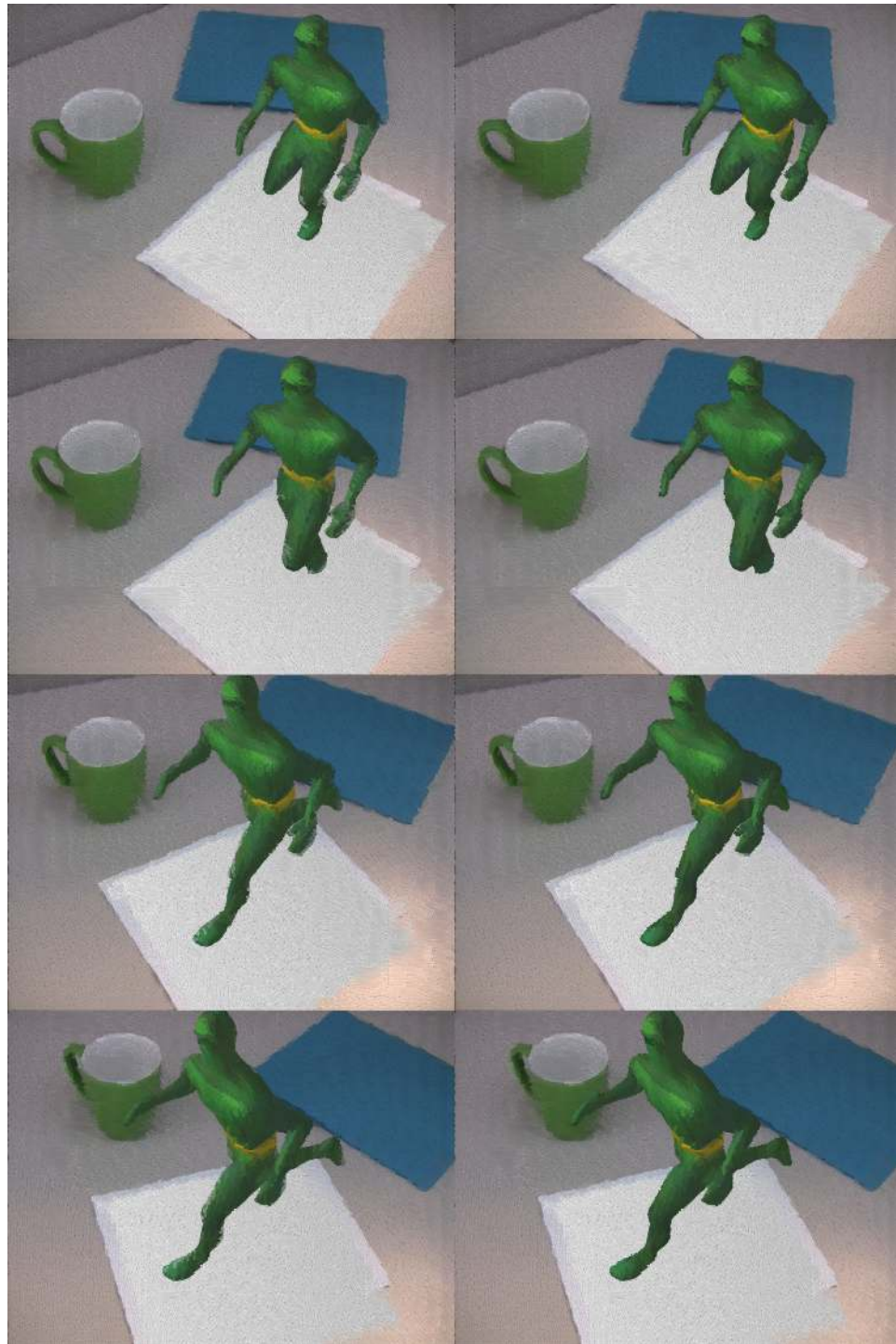
Figure 41: A painted running superhero model. Left: our model space algorithm without edge clipping. Right: the same model space algorithm with edge clipping. Note the artifacts in the images in the left column, including the color bleeding along edges, and incorrect brush stroke movement between frames. These artifacts are removed by using the model information in the right column.
