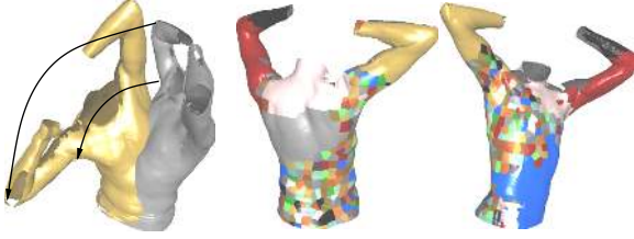
Figure 5: Two views of the clusters color coded on the source surface for the registration example on the left. The registration deforms the source by an almost 180 degree rotation as indicated by the arrows. Many clusters are used in the regions on the lower back and around the arm pit where the source surface bends to align with the target. Large clusters can be used in regions that roughly deform rigidly.
