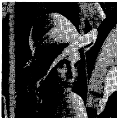
Fig. 14. Data compression using the 4-ring hexagonal filter bank. The entropy of the quantized pyramid was 0.25 bits per pixel for a total of 16 384 bits.
