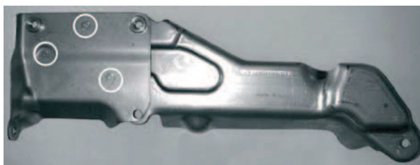
Fig. 10. The reinforcing cross bar made of stainless steel (0H18N9) in the engine chamber of a sport car.
