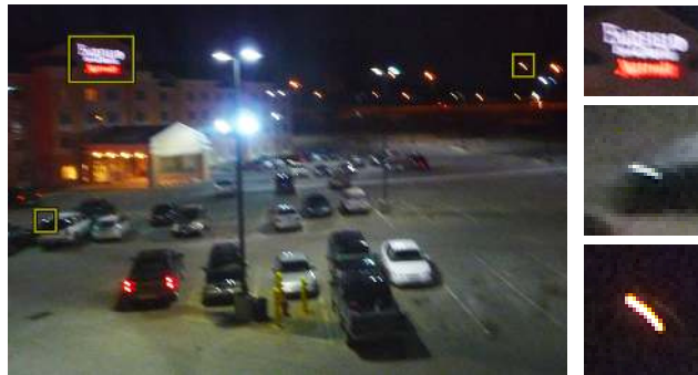
Figure 1. Visible non-uniformity of blur in a shaken image. Left: The blurry image. Right: Close-ups of different parts of the image. Note the differences in shape of the blur between the middle and bottom close-ups.
