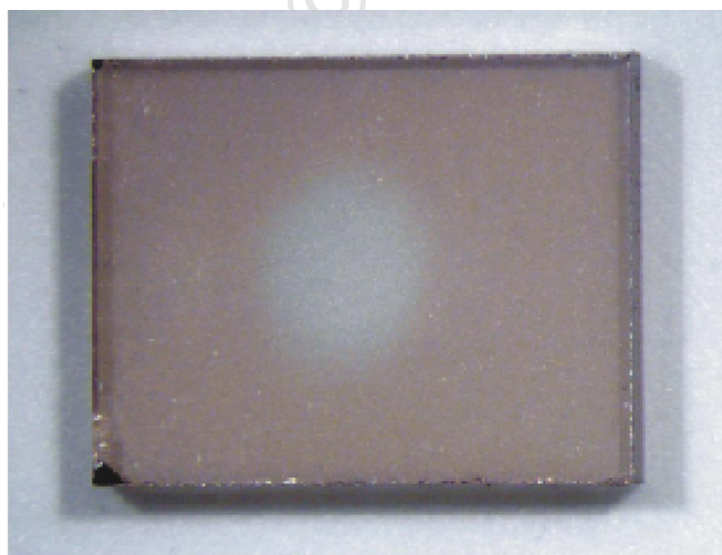
Figure 2 Photo-assisted electron transfer between traps in doubly doped LiNbO 3 . Photograph of a LiNbO 3 crystal (dimensions 5 × 4 × 0.85 mm 3 ) doped with 0.075 wt% Fe 2 O 3 and 0.01 wt% MnO after homogeneous illumination with ultraviolet light (wavelength 365 nm, intensity 20 mW cm -2 , 120 min) and subsequent illumination of the middle of the crystal face with a laser light beam (wavelength 633 nm, intensity 2,400 mW cm -2 , 1/e 2 diameter 1 mm, 30 min). The ultraviolet light excites electrons from manganese into iron, creating Fe 2+ . This centre absorbs visible light and the crystal is darkened. The red light excites the electrons from iron and they are trapped in manganese, where they cannot be excited by visible light. Thus the crystal is bleached by the red light.
